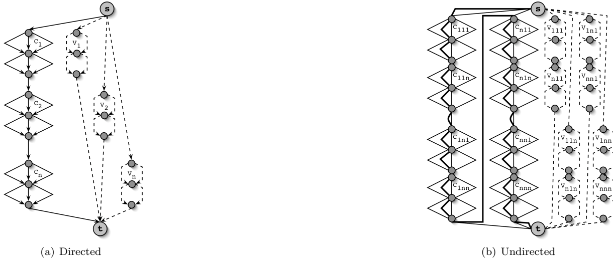
Figure 5: Constructions for non-approximation results for integral max ratio. Both of these constructions paste together the clause and variable components of many copies of the constructions described in Section 3.1. We label clause and variable components of copy x as C_x and V_x , respectively.
