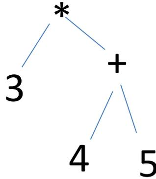
Such a tree has operators in the interior nodes and numbers in the leaves. There is an easy recursive algorithm to compute its value -- evaluate the left child, evaluate the right child and apply the operator to those values.
