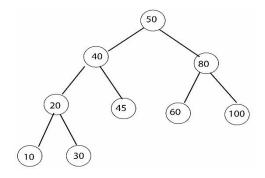
Give either the AVL tree or a level-by-level listing of the AVL tree that results from inserting value 25 into this tree. If you can't easily draw a tree, a "level-by-level listing" of a tree lists the root on the first level, all of the children of the root on the second level, the grandchildren of the root on the third level, and so forth. A level-by-level listing of the tree shown is
