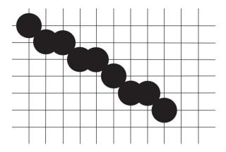
**Pitteway**: Start with  $d_0 = \frac{1}{2}$ . At each step, if  $d_i \ge m$ , choose  $y_{i+1} = y_i$ ,  $d_{i+1} = d_i$ -m. On the other hand, if  $d_i \le m$  choose  $y_{i+1} = y_i + 1$ ,  $d_{i+1} = d_i + 1$ -m. You can take the value of d as the intensity for a white polygon drawn on a black background; use 1-d for a black polygon on a white background.
