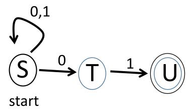
This is called a "Nondeterministic Finite Automaton", or NFA because in state S there are two options on input 0: we can stay in state S or transition to state T.
